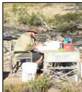
Sampling for aquatic macroinvertebrates using a sweep net and picking live bugs on the river bank
