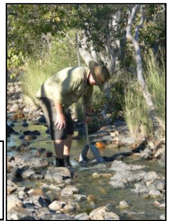
Sampling for aquatic macroinvertebrates using a sweep net and picking live bugs on the river bank
